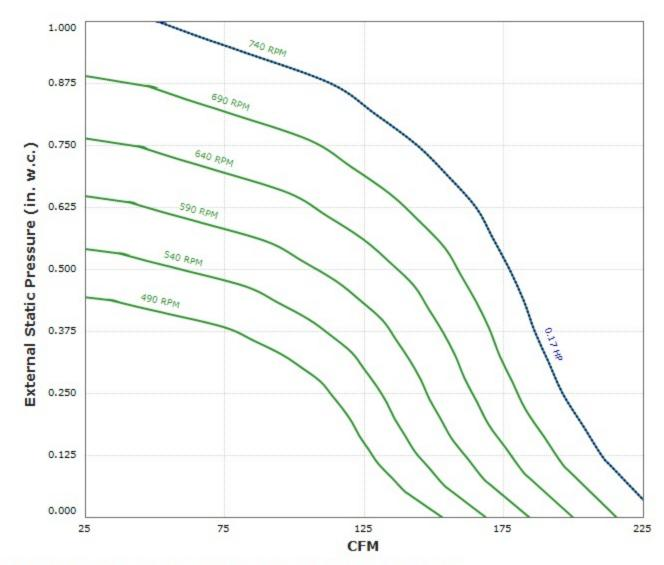
Max Sizeable RPM = 740 RPM. Curve shown extended beyond this point for reference only. Motor Broan 127 W, 120V has an rpm range of 444 to 740.
